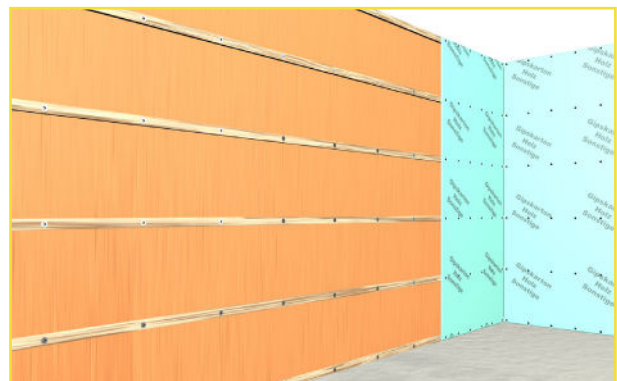
Fig.16: Fixed fastening of the sheets with the help of the battening - Removal of the auxiliary fastening
